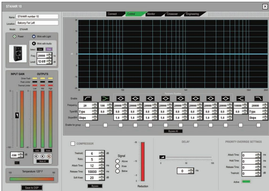
The RHAON Module’s DSP is designed for “technical” or “corrective” functions. 8 bands of parametric equalization are available, along with high and low cut filters and high and low shelving filters.
