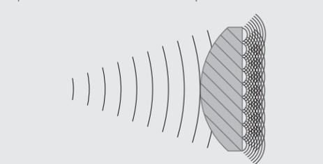
At lower frequencies the refractor lens represent a closely spaced array of diffraction slots.
