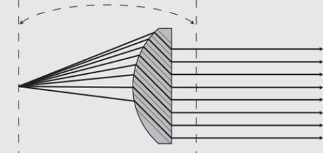
The higher frequencies pass through the device as "rays".
