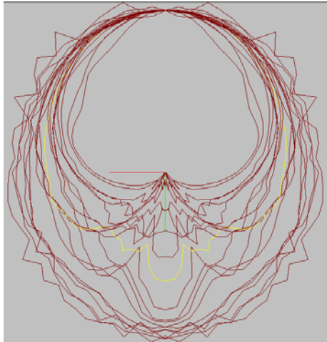
The polar response of the Iconyx co-axial 4-inch driver: high frequency dispersion is much wider. The off-axis narrowing observed in many coaxial transducers is absent, thanks to a time-aligning passive crossover network.
